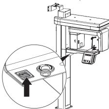
The main power switch lights up green after it is switched on. The status LED lights up blue.
