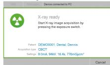
Trigger the image by pressing and holding the button on the exposure switch until the acoustic signal stops and the control lamp goes out. The scan times depend on the patient type, imaging program and image quality (see "12 Program parameters").
